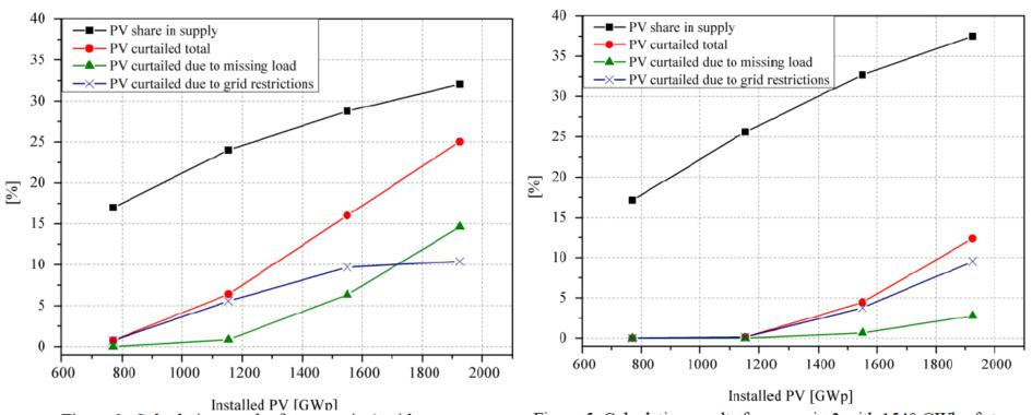
Figure 3: Calculation results for scenario 1 with no storage
